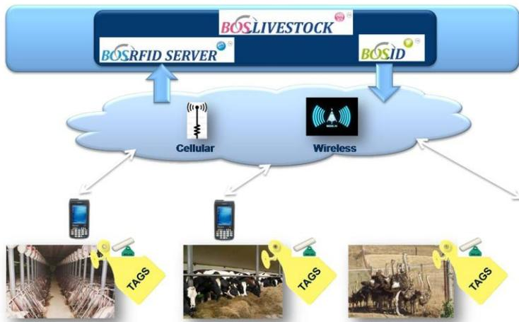
Every animal entered into BOS Livestock is assigned a unique identification number, as a way to positively identify an animal. Farmers or herd managers use handheld terminals with integrated RFID scanners to enter and collect the data, and data is synchronized when the terminals communicate with the management program, which is built upon the browser-based BOS ID platform.
